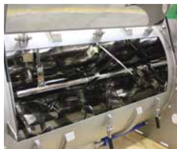
304L / 316L stainless steel chamber internally polished
